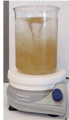
Sediment and water in a beaker on the mixing apparatus. Too much mixing causes air bubbles, too little mixing provides poor suspension.
