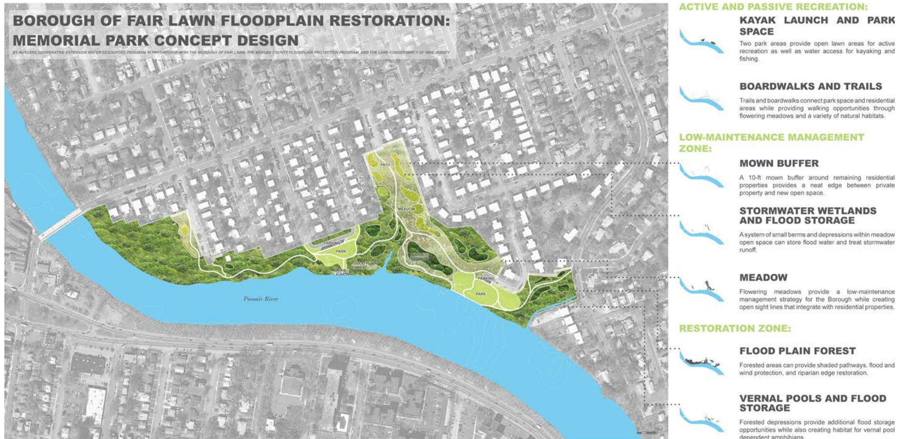
Figure 9.3 Fair Lawn Floodplain Conceptual Restoration Plan Conceptual plan for establishing a flood resilient landscape in a former residential section of Fairlawn. The preliminary design outlines areas for a variety of appropriate habitats as well as trails and open space amenities. Such conceptual plans provide a long-range vision of the landscape transition from inhabited neighborhoods to open space and identify areas where flood storage interventions are most feasible. (Credit: Rutgers Cooperative Extension)
