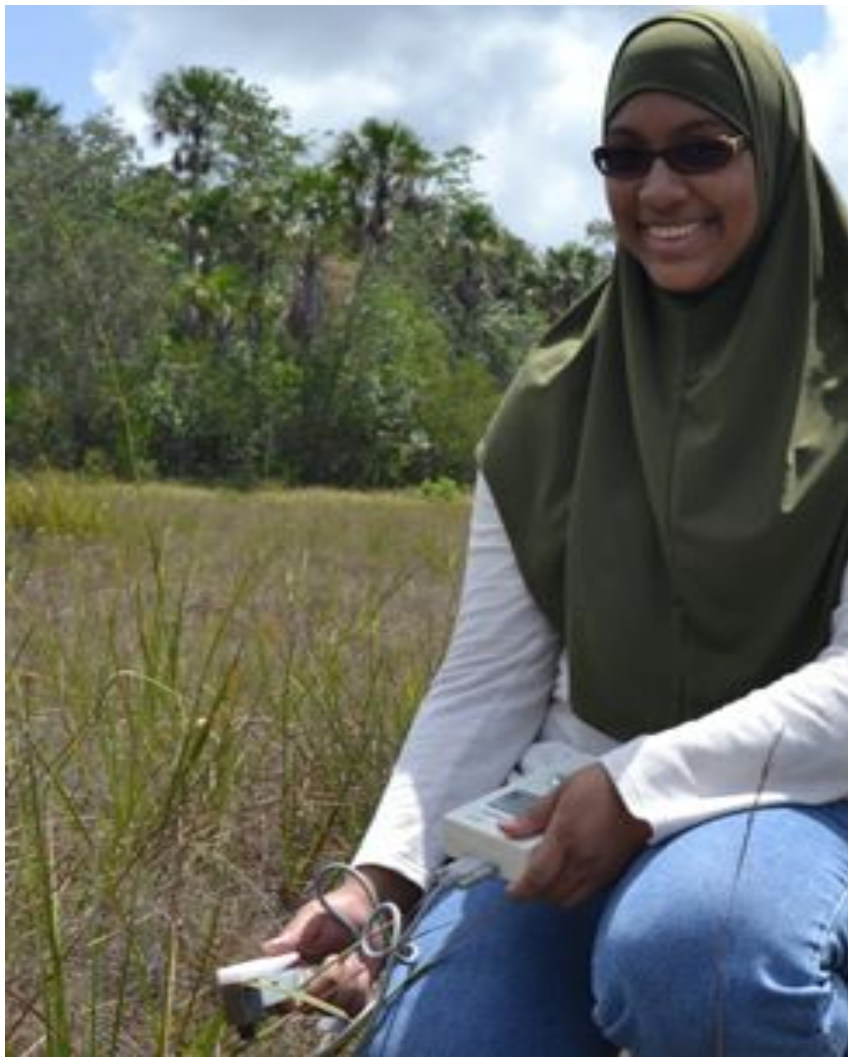
A Porometer (SC-1 Decagon Device) being used in the field to measure transpiration
