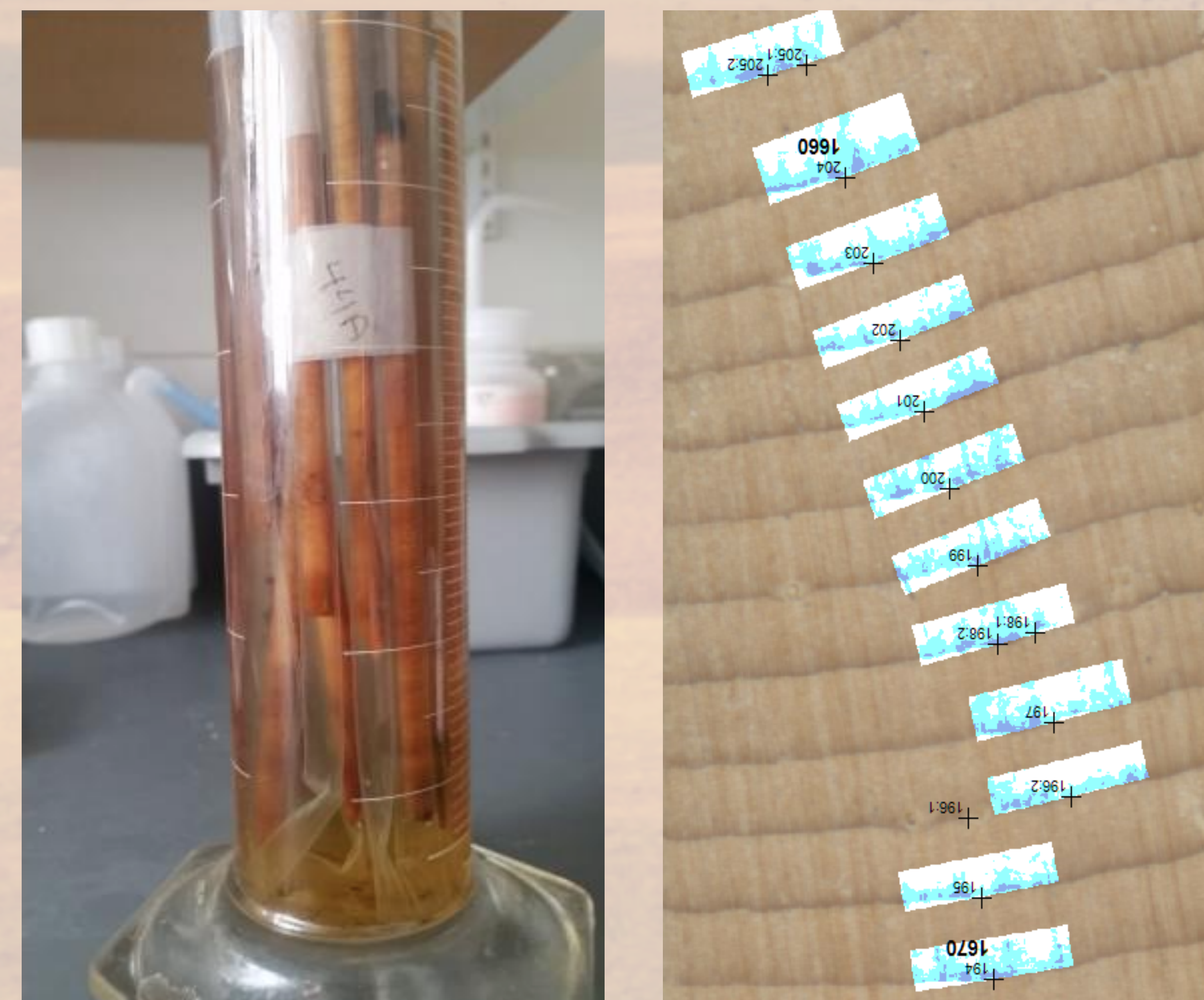
Figure 2A. Tree cores in an acetate bath for extraction. 2B. A screenshot of blue light reflectance performed on a high resolution core scan. The blue band represents latewood density values extracted from image analysis.
