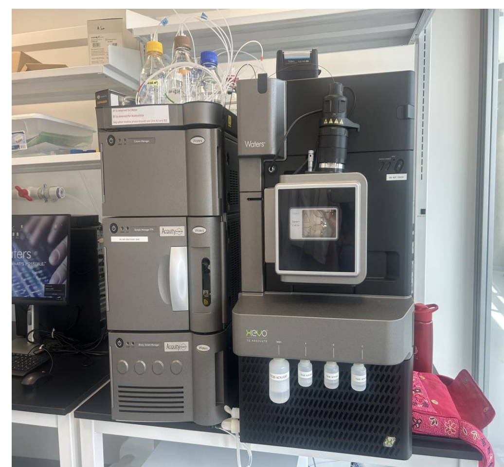
Figure 3. Lab equipment: Liquid chromatography-mass spectrometry (LC-MS) machines.
