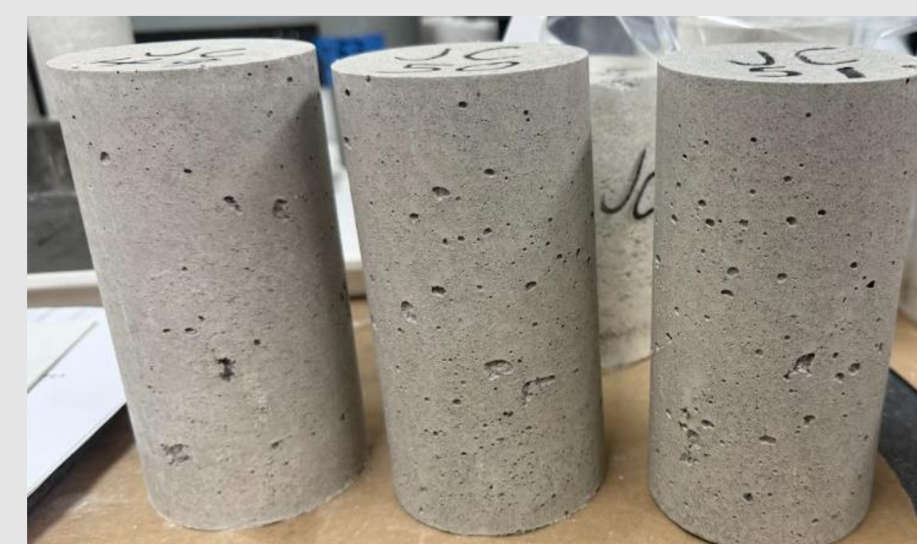
Figure 1: Cast Cylinders of Wollastonite and concrete rubble.
