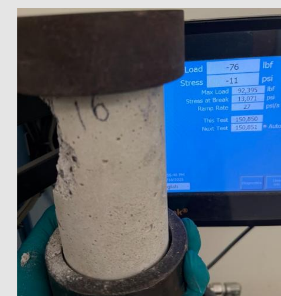
Figure 3 and 4: Compression tested cylinders.
