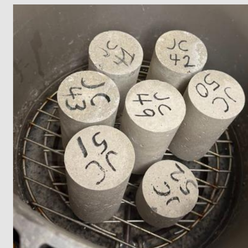
Figure 2: Cylinders in carbonation chamber.
