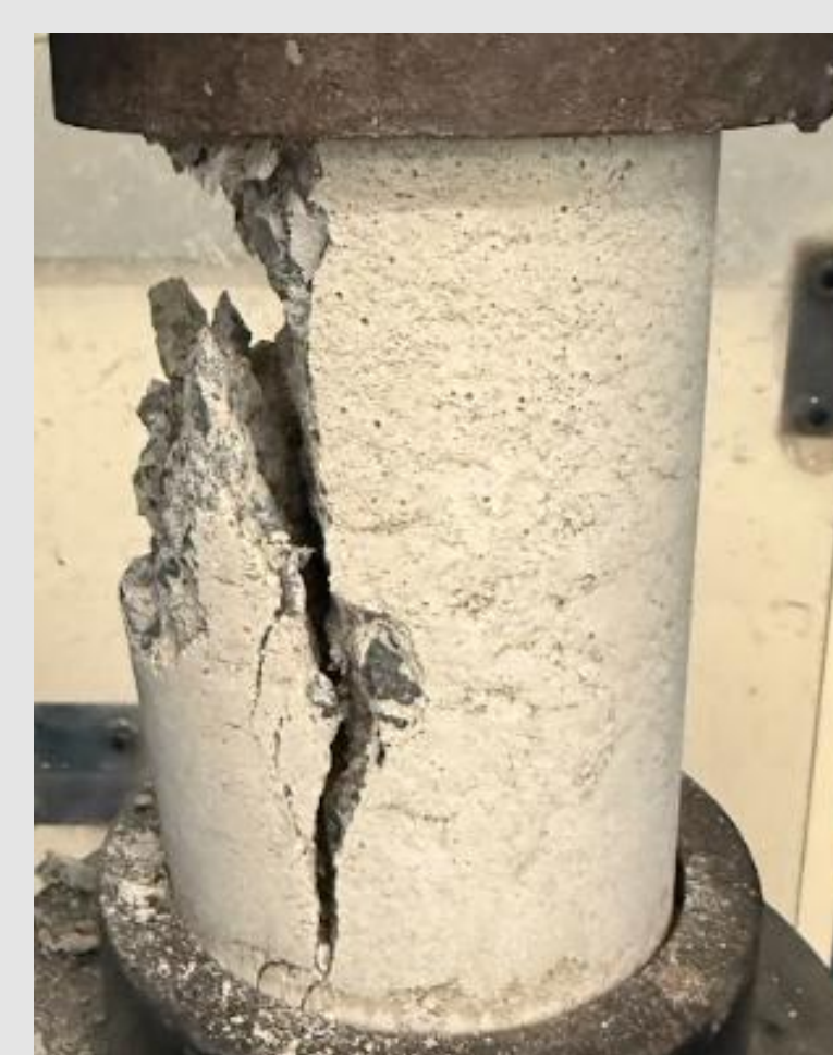
Figure 3 and 4: Compression tested cylinders.
